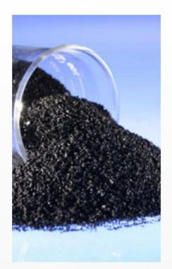
Activated Carbon is used to remove pollutants from air or water streams, both in the field and in industrial process such as spill cleanup, solution to groundwater management, drinking water filtration, air purification and wash out volatile compounds.
